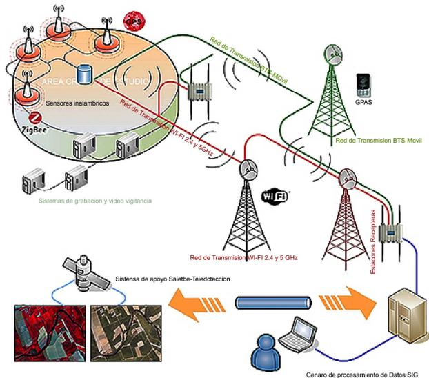
In each sensor node, the sensor data deposit to a fuzzy algorithm for fire detection. This algorithm makes that we use all the sensors capacity proportional to its influence in the region and distinguish the fire. By this work, error rate detection becomes low and fire can be detected with high certainty.
