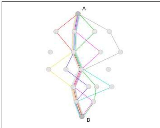
Maybe due to the passage of time and the use of a commute, its battery power on that path declines and it is not the good path for sending and receiving. It is therefore important that algorithm always consider the energy consumption of the selected route. Figure 7 clearly illustrates this issue.
