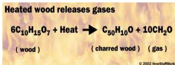
This gas ( $10CH_2O$ ) that is created by the reaction of wood and heat, subjected to the atmospheric oxygen ( $O_2$ ) exhibit luminescence to gas ( $H_2O$ ,  $N_2$ ,  $CO$ ,  $CO_2$ ).
